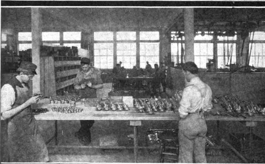
Part of the Space Devoted to Testing, Showing Lots of Model L & F Carbureters Undergoing Final Inspection
